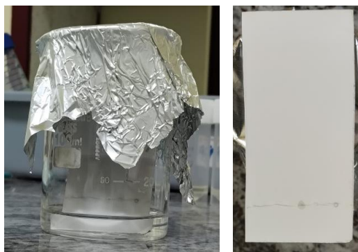
Fig: 3 TLC Chamber and Silica gel Plate
