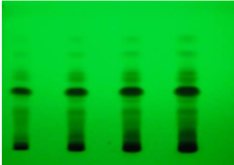
Figure No 1: High-performance thin-layer chromatography chromatograms of Spermadictyon suaveolens root and standard for Quercetin under UV at 365 nm
