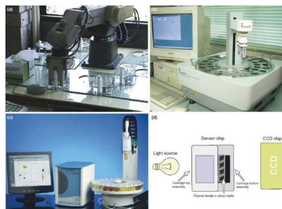
Fig. 8: Commercially developed and developing taste sensors. (a) Taste sensor SA401 developed by Anritsu Corp. (b) Taste sensor SA402B developed by Intelligent Sensor Technology (Insent Corp). (c) Astree electronic tongue developed by Alpha M.O.S. (d) a schematic of the electronic tongue developed by the University of Texas and usion.
