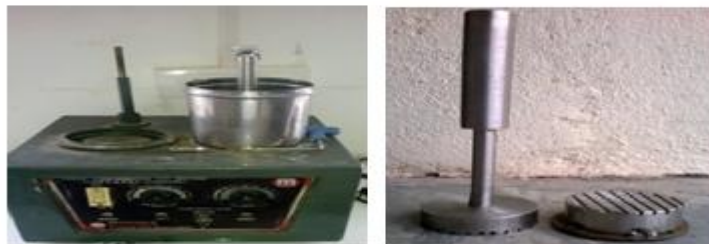
Fig. 4: Lab fabricated medicated chewing gum apparatus with S.S Die and punch.
