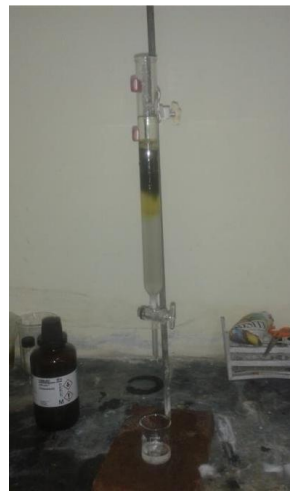
Figure 5: Column chromatography Ethanol and Petroleum ether crude extracts
