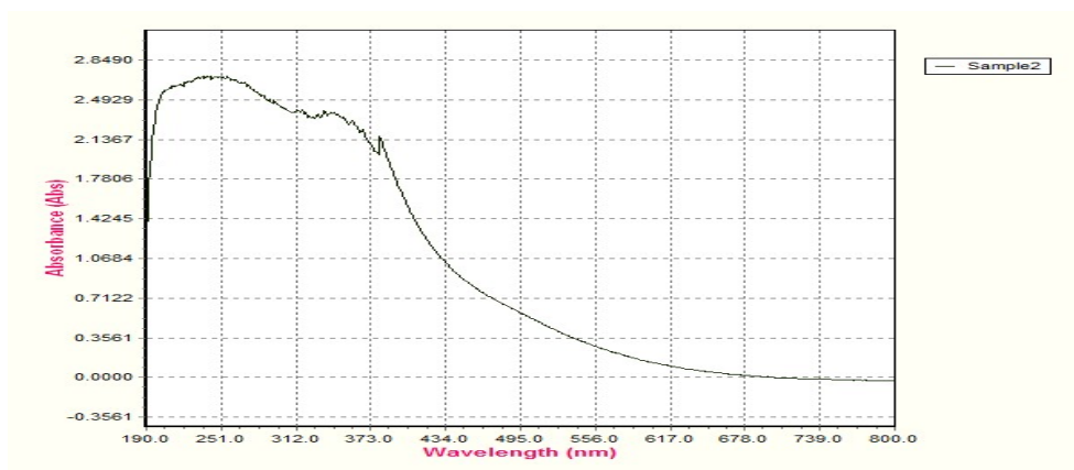
Fig. 3. Electronic absorption spectra of Co (II) complex of chalcone of 5-methyl furfural.
