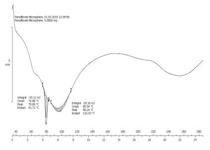
Fig. 8. DSC analysis of Fenofibrate microspheres.
