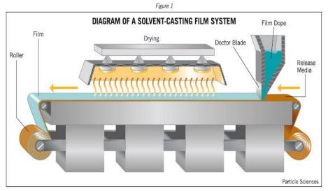
Fig. 6. Description of solvent casting technique.
